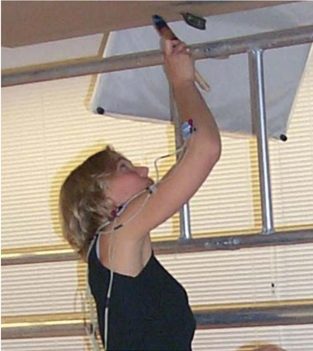
**Fig. 15.2** Electromyograph measurements.
